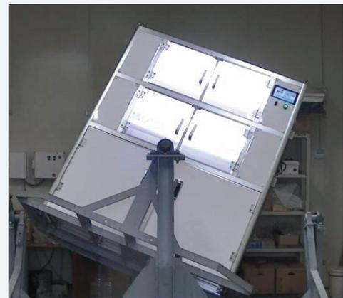
Rolling and Pitching tests at 22.5 degrees have been conducted.
